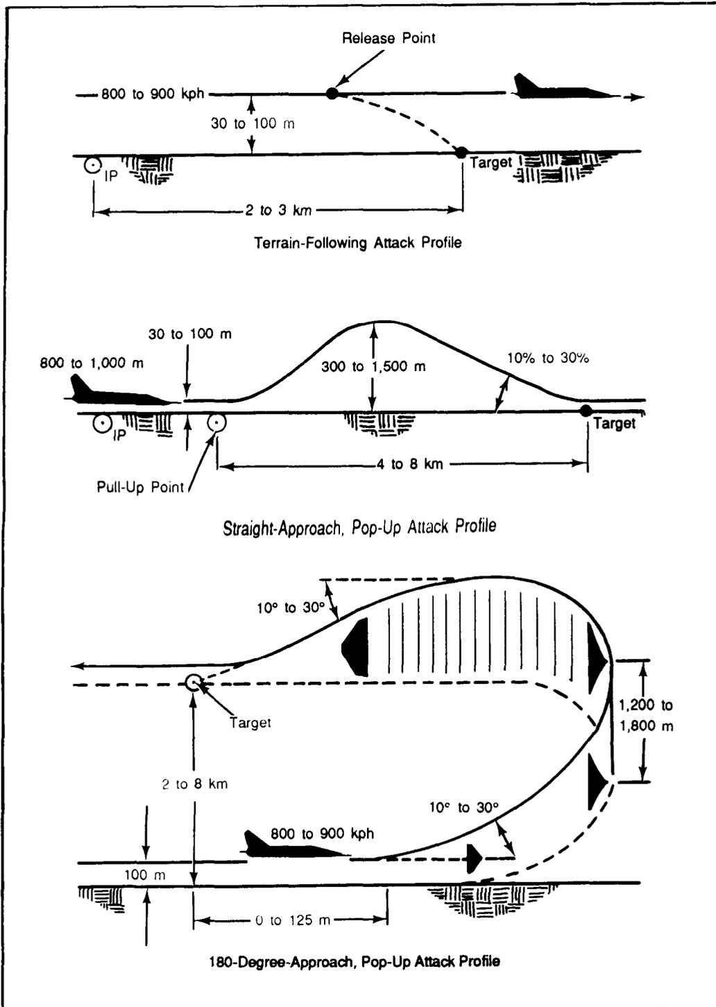
Figure 7-2. Typical Aerial Attack Profiles Against Fixed Facilities
